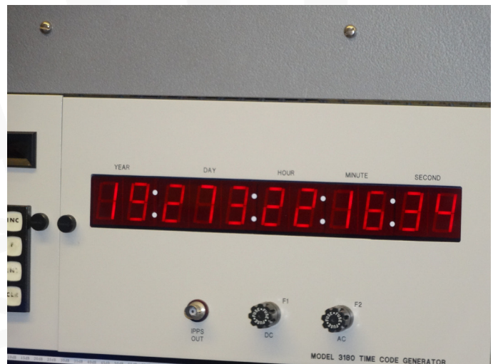
Capturing the Exact Time of our visit - one of WWV's redundant Time Code Generators.
