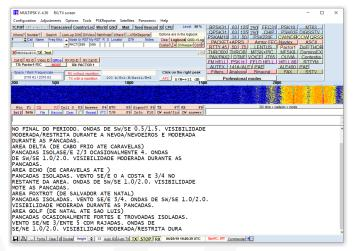
Figure 5: MultiPSK Decoding a Pactor Transmission
