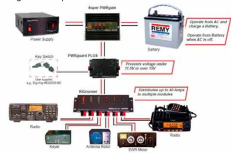
This set-up connects PWRguard PLUS input to the Super PWRgate PG40S output terminal and then plug the PWRguard PLUS output into the RIGrunner input terminal. This will provide protection for the battery and all the devices that are plugged into the RIGrunner. Additionally, after loss of AC mains power, the PWRguard PLUS will reset the system after the power is restored.
