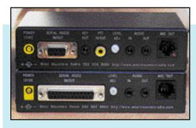
Rear view of the RIGblaster (bottom) and RIGblaster Plus (top) show additional jacks added on the Plus version. See text for details.
