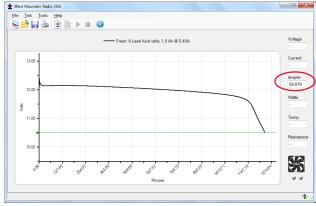
**EXAMPLE:** We purchased a 60Ah battery and should expect the graph to show the battery to be around 60Ah. Since our test verifies this capacity, the battery is good to use in our UPS.
