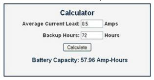
The required battery capacity would be 58 amp-hours.
